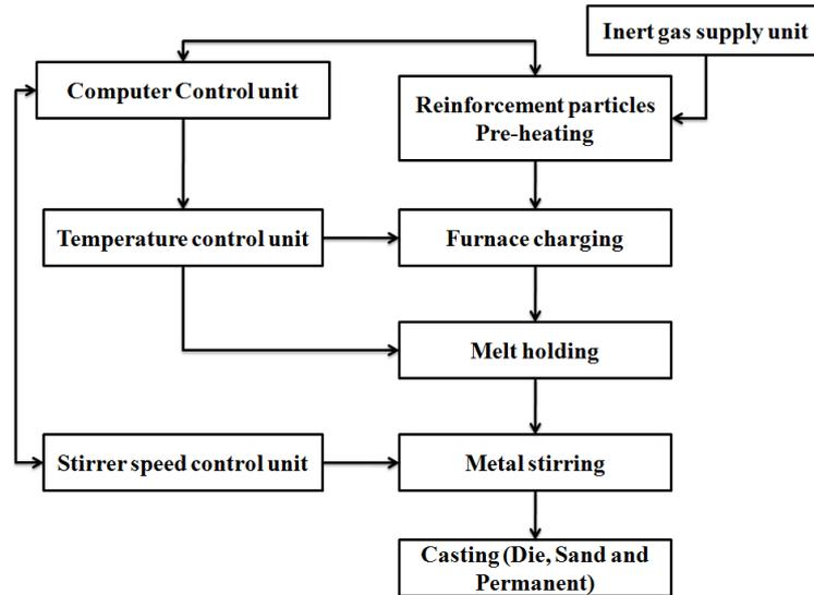
**Figure 2.1.1: Flow Chart of Stir Casting Process**
