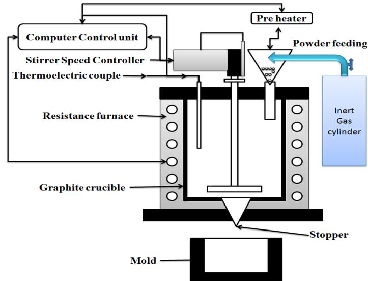
**Figure 2 1: Schematic of Stir Casting Design Setup**
