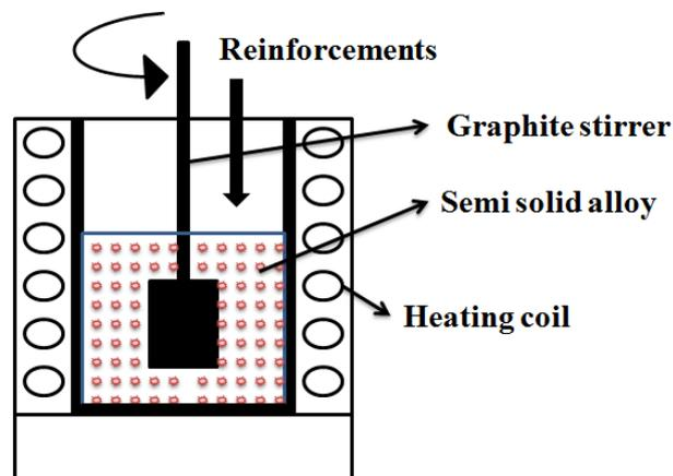
**Figure 2.2: Design Setup of Compo Casting**
