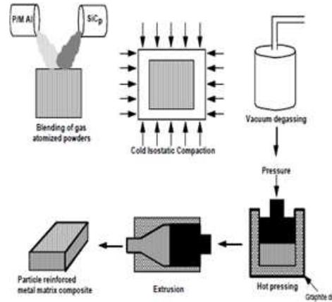
**Figure 2.4: Schematic of Processing of Powder Metallurgy [38]**
