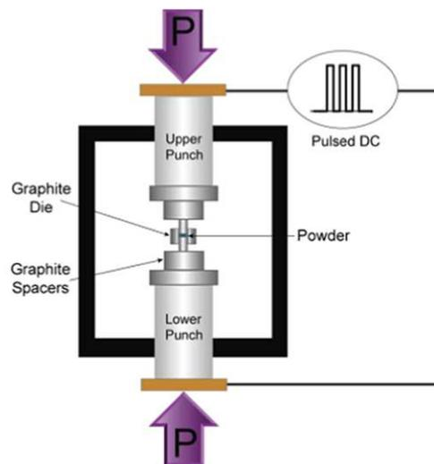
**Figure 2.10: Schematic of the Spark Plasma Sintering Apparatus [76]**
