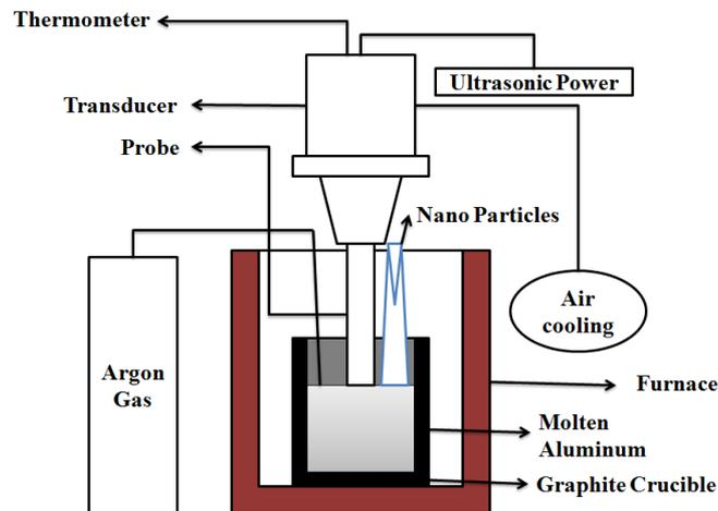
**Figure 2.8: Design of Ultrasonic Assisted Casting Process**
