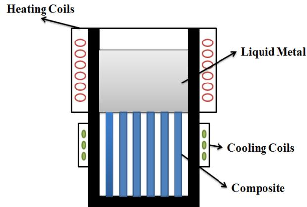
**Figure 2.6: Process of in Situ Synthesis**
